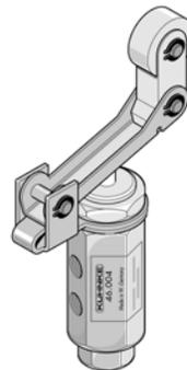
Roller lever operates valve only in one direction. Can be used for limiting travel on machinery. Actuator travels and force, same as 46003. Weight: 5.1 ozs. Dimension above valve body is 1 1/2".
