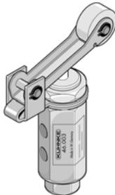
Used as pneumatic limit switch or position detector. Actuator travel 5/32" for valve operation. Actuation force approx. 1.3 lbs. Weight: 5 ozs. Dimension above valve body is 7/8".
