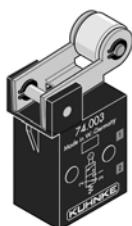
Used as pneumatic limit switch or position detector. Actuator travel 11/64" for valve operation. Actuation force approx. 2 lbs. Weight: 2 ozs. Dimension above valve body is 11/16". Body mount.
