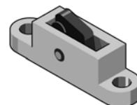
One way trip mechanism can be used with plunger or ball operated valves. In one direction, mechanism forces ball to actuate valve. In the opposite traveling direction, mechanism is forced into base offering no resistance for valve switching. Tripping mechanism travel into base is 5/64". Overall dimensions: 1 1/8" L x 1/4" W x 3/8" H.
