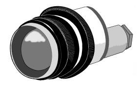
AL indicators provide a 2 color visual indication of the presence or absence of air pressure in a system. The indicators are available in a variety of color choices. The AL series are fixed 2 color units that change color when air pressure is applied.
