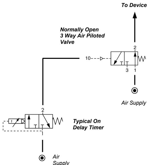
On delay timer signals can be converted to an off delay signal with the use of an interposing normally open 3 way air piloted valve.
