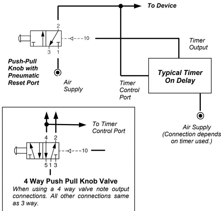
Push-Pull valve can be used to start and stop system manually while providing timing to the circuit. A 4 way valve can also be used when operating a double acting cylinder, or for alternating outputs.
