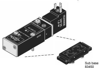
The Series 83 sub base mounted valve provides a simple answer to miniature 5/2 valving. The valve is constructed of a moulded body and utilises O-ring construction to provide a lightweight, durable alternative. The valve has red pop-up indicators to show position, as well as a manual override and an external air pilot supply port connection, used when switching pressures less than 2.5 Bar.
