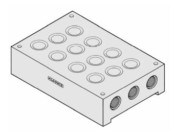
Manifold kits for 1/8 ported Series 87, 5 way valves include a manifold with 1/4 supply ports at each end, and valve mounting hardware. Standard manifolds are available for 2, 3, 4, 6, or 8 station configurations. Manifolds can also be custom made with any number of stations; consult factory for details. These units cannot be used with old design valves using 22mm solenoid coils, see valve catalog page.
